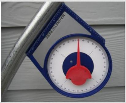
The last few bends will be tough, use a cheater bar as needed. This should be as tight a fit as possible to go into the end of the EMT. You do not want to collapse your EMT, or elongate the EMT opening
