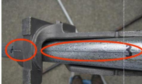
Pull gradually on the EMT to meet the 5 degree mark on the bender
